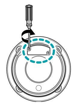
Make sure that the cover is joined properly when screwing it; otherwise, the IP67 level is not guaranteed.
