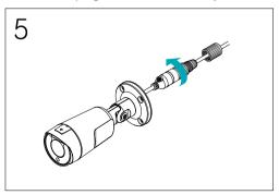
Push the waterproof cap body and cap into the RJ45 jack and rotate it.
